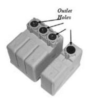
6. Reinsert the cartridge leaving the transparent tape on the outlet hole(s), see general tips, and run 1 - 3 cleaning cycles as per printer instructions. If necessary leave cartridge in printer for up to 24 hours to allow ink to flow to the print head.
